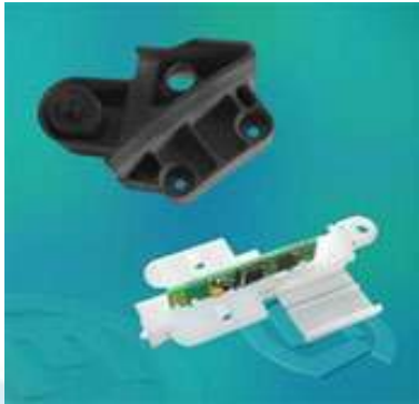
图：磁体和3D霍尔传感器集成电路
