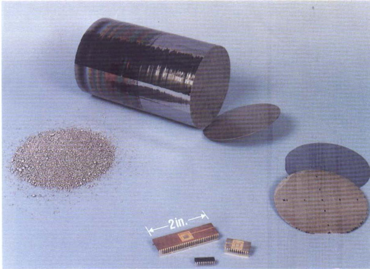
**Figure 23.26** Elemental silicon. To prepare electronic devices, silicon (powder, left) is melted, drawn into a single crystal, and purified by zone refining. Wafers of silicon, cut from the crystal, are subsequently treated by a series of elegant techniques to produce various electronic devices. (Courtesy of Texas Instruments)
