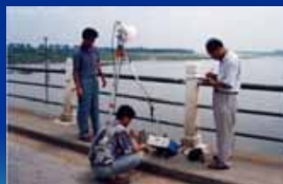
Flow measurement is made with electric wave current-meter
