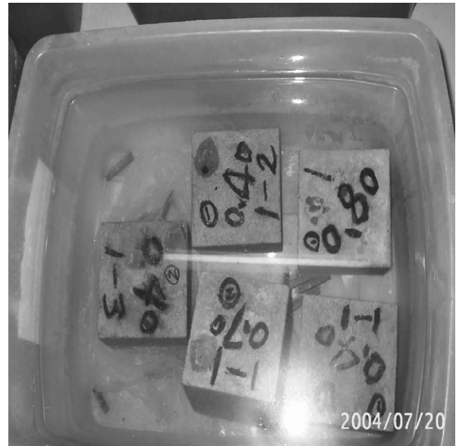
Fig. 1. Specimens are immersed in sulphate solution.
