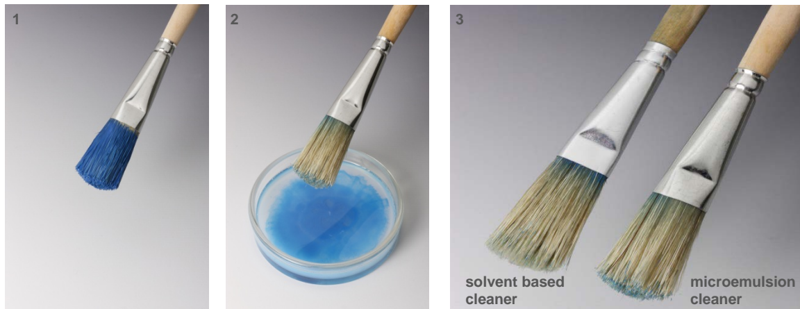
Fig.1: Brush cleaner test with an off-the-shelf brush cleaner, containing large amounts of volatile solvents (photo 3, left) and a cleaner based on the microemulsion developed at the Forschungszentrum Jülich (photo 3, right).
