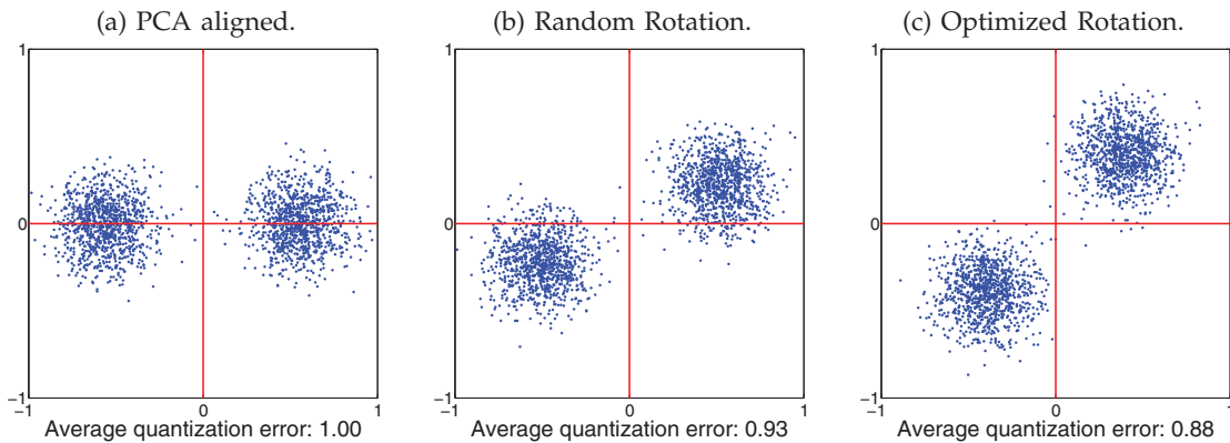
Figure 1. Toy illustration of our ITQ method (see Section 3 for details). The basic binary encoding scheme is to quantize each data point to the closest vertex of the binary cube, (\pm 1, \pm 1) (this is equivalent to quantizing points according to their quadrant). (a) The x and y axes correspond to the PCA directions of the data. Note that quantization assigns points in the same cluster to different vertices. (b) Randomly rotated data – the variance is more balanced and the quantization error is lower. (c) Optimized rotation found by ITQ – quantization error is lowest, and the partitioning respects the cluster structure.
