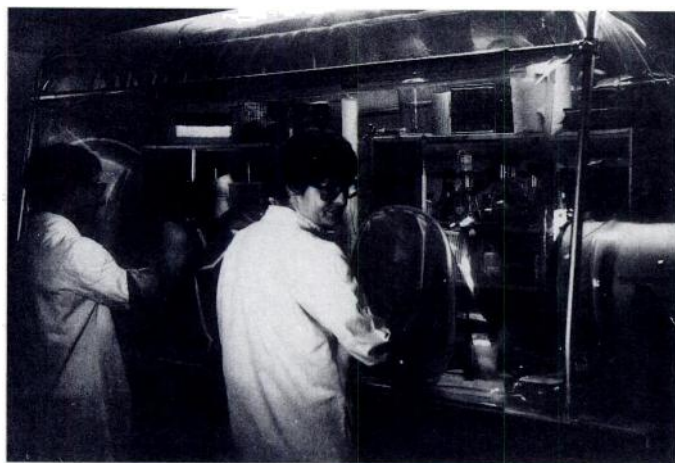
Figure 5. Steve Ragsdale and Ewa Pezacka isolating oxygen-sensitive enzymes from C. thermoaceticum by use of an anaerobic hood.
