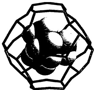
Figure 3. TMA + cations occluded into the sodalite cage (cage \beta ). In this scheme, the network-forming elements T (T = Si, Al, ...) are located at the corners, defined by the intersection of three edges. O atoms can be found at the center of each edge.
