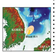
June 2007 piston coring in the East Sea confirmed the presence of gas hydrates
